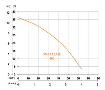
Shaft Speed: 2850 rpm Outlet: 50mm, 2in
